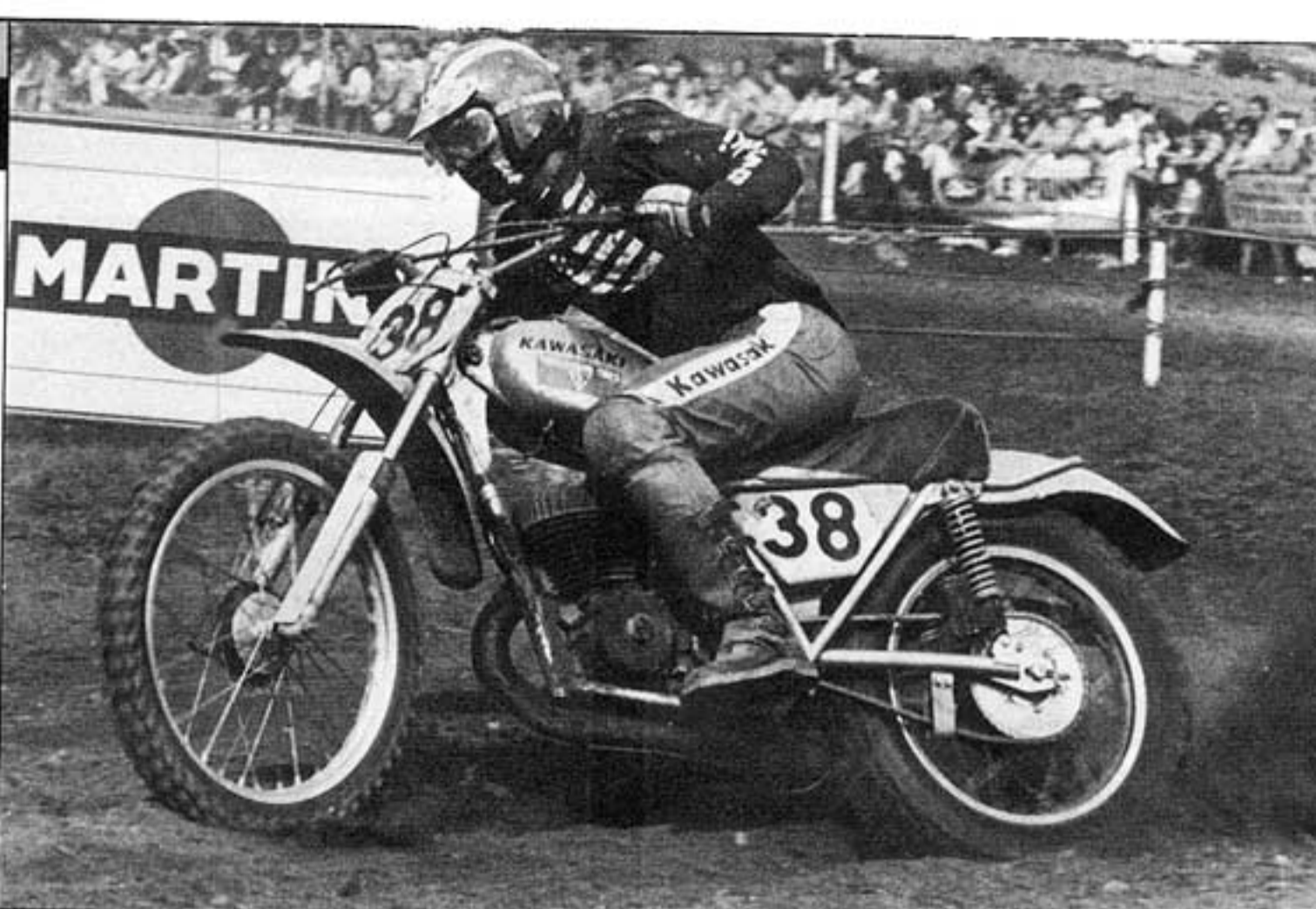
"Grand Prix action at Luxembourg in '73. Those are Koni shocks with oil-cooler bodies, Betor forks with a Bultaco front wheel, British aluminum tank; it was a 450, and we were semisupported, with Steve Johnson working on the bike."
