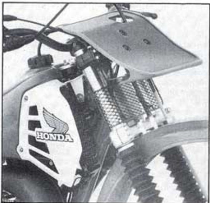
Air flows beneath plate to twin coolers Reshaping the gas tank for a lower cg.
